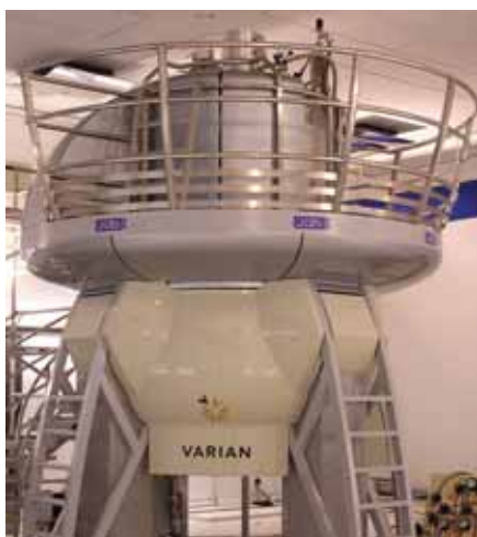
Above: the 900 MHz magnetic resonance spectrometer which is five metres tall and cost £3.5 million Right: The Smyth family
